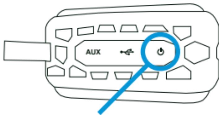
Slide the rubber flap sideways to expose the power switch.
