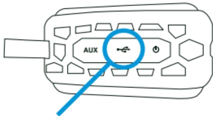
To charge, plug the supplied USB cable into the VIVID and the other end into a computer or 5V/1000mA charger.
